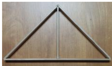
Fig. 7: 45^\circ roof structure model
