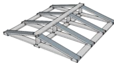
Fig. 2: Initial roof frame model with rafters, studs, ridge board, and ceiling joists
