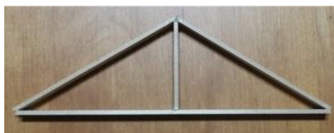
Fig. 6: 30^\circ roof structure model
